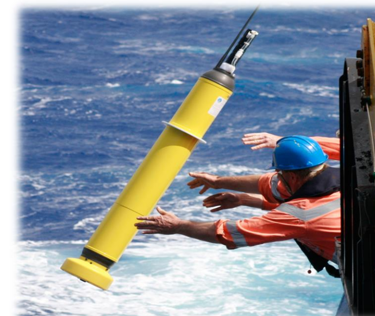
Figure 8: By NOAA Research News. An Argo float being deployed from a boat.
